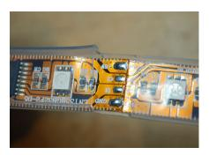
Press the soldering iron against the four joints while pulling the two pieces apart:
