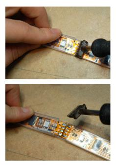
Cut the remaining rubber underneath with scissors:
