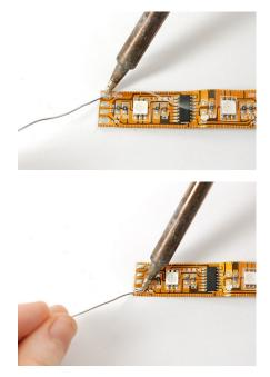
Start by soldering a red wire to the +5V power line:
